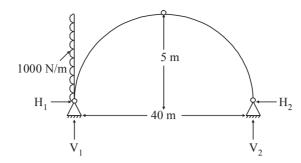
Considering right segment and taking moment about crown :  $H_2 \times 5 = V_2 \times 20$
